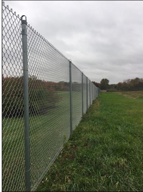
**Photo 5:** View of the airport perimeter fence along West Hammer Road. Note that the bottom of the fence is not flush with the ground, which enables small- and medium-sized mammals to enter the AOA.
