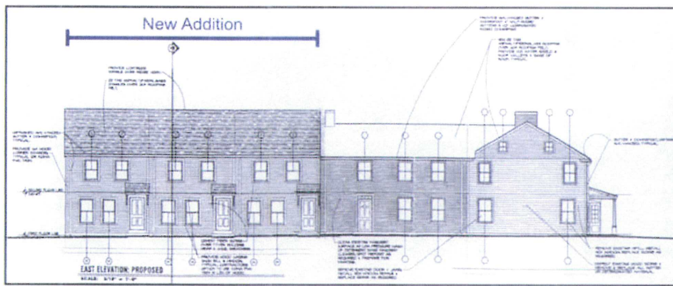
Figure 16. The proposal to add three row houses to the rear ell of this early-19th century residential property doubles its size and does not meet the Standards.
